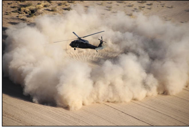
Figure 5. Army UH-60 Black Hawk helicopter in enveloping dust cloud (brown-out) (U.S. Army photo)
