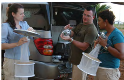
Figure 2. NAMRU-3 and NEPMU-2 personnel deploy ultraviolet light traps in Liberia to monitor for Anopheles gambiae species mosquitoes
