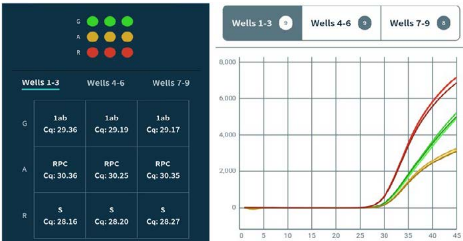
FIGURE 2a. Portable Multiplex RT-PCR for Wastewater Sample Screening and SARS-CoV-2 Detection a
